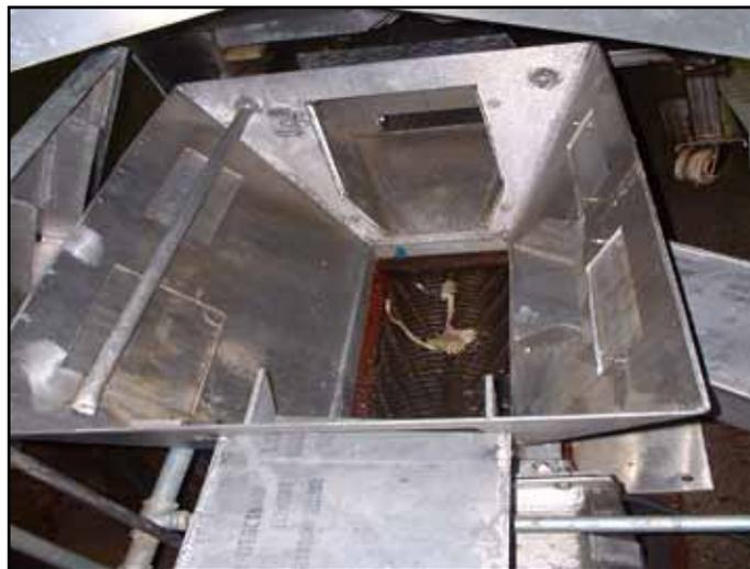
*Monsters readily grind up the many types of seafood remains conveyed into its specially designed cutter teeth.*
